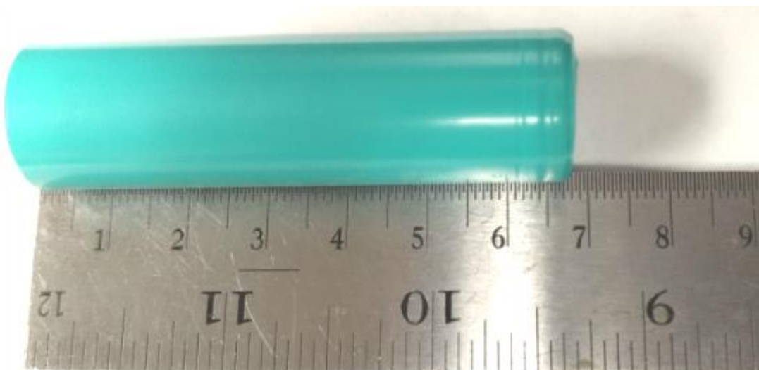
Figure 4- 1: INR 18650-20R Li-ion cell captured from CALCE website [63]
